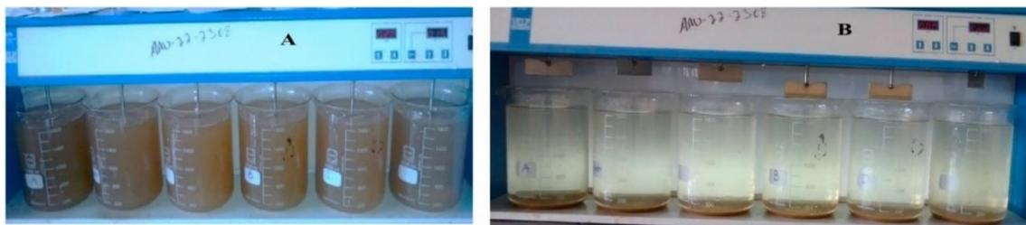
Fig 5: Sample A- untreated water and Sample B- water treated with different Natural Coagulant samples.
